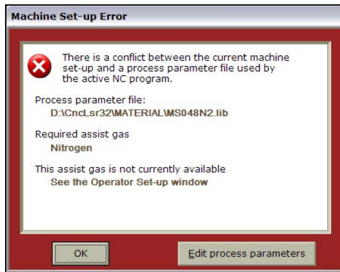
Machine setup error resulting from an assist gas conflict.
